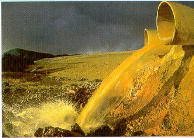
FIGURE 11.7 Pipe discharging partially treated effluent from the Climax Molybdenum Mine in Colorado. (1993, National Geographic 184(5A):77.)
