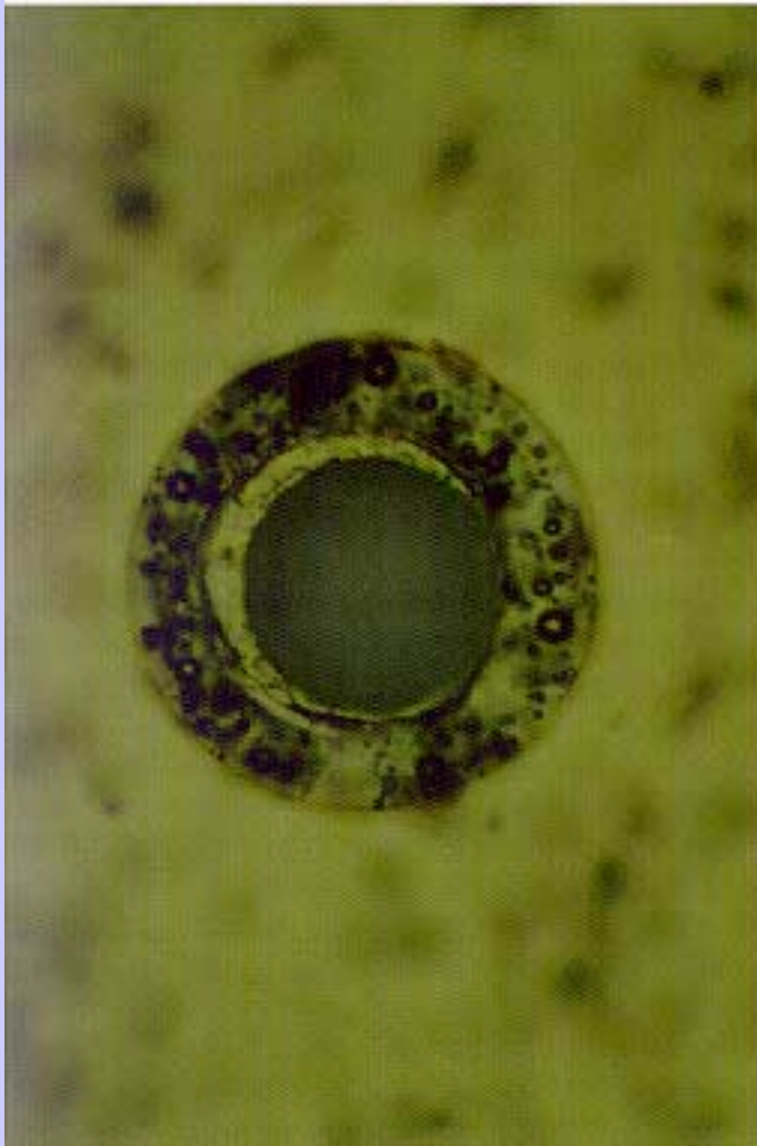
Photograph of hollow glassy fly ash particle (0.01 cm D)
